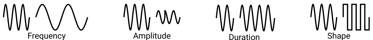
Figure 1.3 – Four parameters of the vibrotactile output vocabulary: frequency, amplitude, duration and shape.
