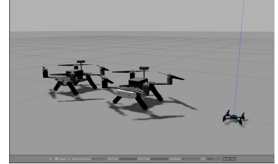
Figure 3.1: Two Intel Aero UAV and one Crazyflie drones simulated in Gazebo. Courtesy of Vincent Le Doze.
