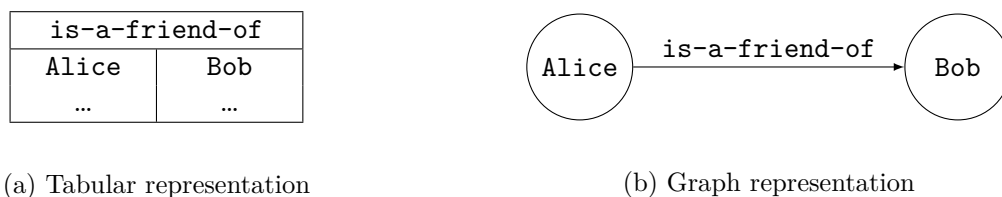
Figure 1.1: Two possible representations of relational data illustrated with the fact “Alice is a friend of Bob”. In the tabular representation, the table corresponds to the relation is-a-friend-of and each line corresponds to an instantiation or an assertion of this relation between two specific entities (here, Alice and Bob ). Alternatively, in the graph representation, each assertion is represented as an edge labeled by the relation between two nodes representing the entities.
