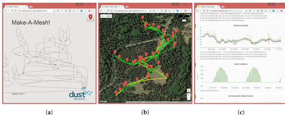
Figure 6.3: The SnowHow networks. (a) logical view of the topology, (b) location of the nodes, (c) sensor data received live from the field. Taken from [165].
