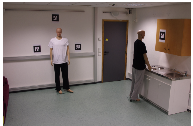
Fig. 2. View of the experimental room. The room is designed to simulate a real living apartment. Some augmented reality tags have been placed around the two dummies.
