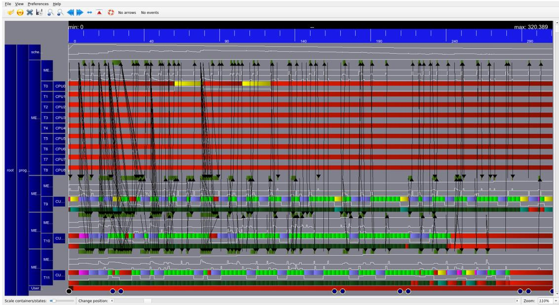
Figure 3.30: Gantt chart visualization of an execution trace.
