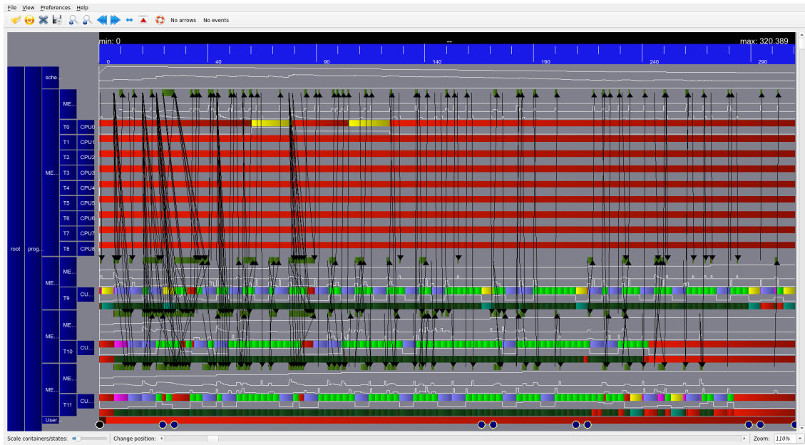
Figure 3.30: Gantt chart visualization of an execution trace.
