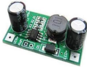
Figure 4.10: DC to DC Step-down 700mA current driver
