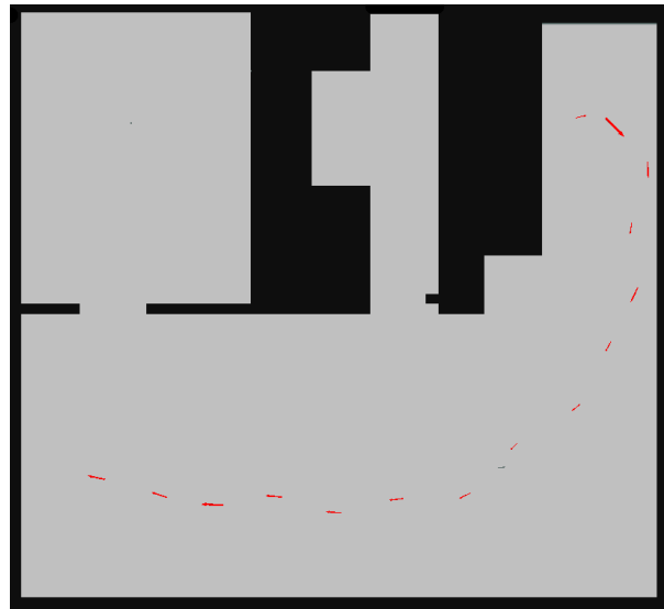
Figure 3.16 – Extraction of footsteps by tracking the evolution of the center of mass of a person using the load-sensing floor. The steps are overlaid on a 2d top view of our prototype apartment.
