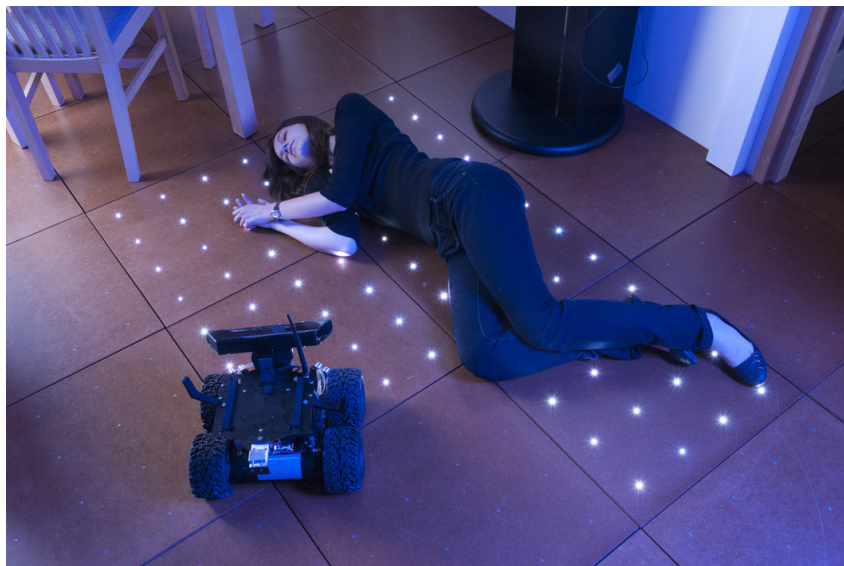
Figure 9.2 – Investigating the health state of a person using a mobile robotic actuator, after a fall detected by the sensing floor.
