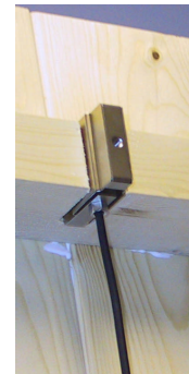
(b) An enlarged view of the load cell supporting the floor.
