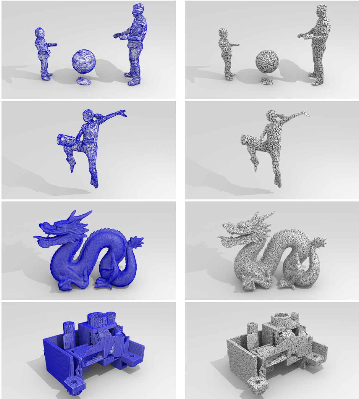
Figure 13: More examples of clipped (non Centroidal) Voronoi diagrams. Left: input triangulations. Right: clipped Voronoi diagrams.
