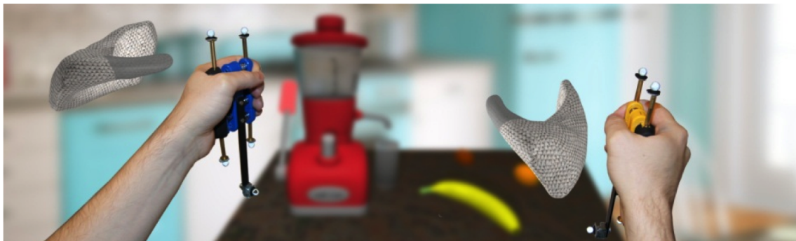
Figure 9.1 – Illustration of the Virtual Mitten. Each hand holds an elastic device to control a corresponding virtual mitten (in gray) and to grasp virtual objects in a bimanual scenario. The grip force applied by the user is measured to generate pseudo-haptic feedback.
