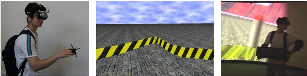
**Figure 10.1** – The Magic Barrier Tape displays the boundaries of the real workspace as a virtual barrier tape, and uses a hybrid position/rate control to travel in the VE. The user (left) “pushes” on the Magic Barrier Tape (center) to move inside the VE when he reaches the workspace boundaries. Any tracked body part can be used to trigger the Magic Barrier Tape (right).
