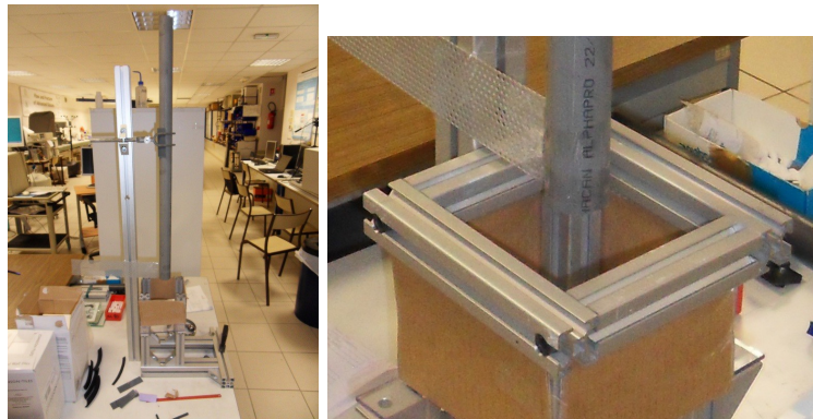
Figure 2.7 – One of the test benchmark we designed for our validation experiments. Left: overview of the bench, a ball is dropped in the tube to fall on a tile set up on its support. Right: zoom on the aluminum support of the tile. To design a 4 punctual contacts test, 4 metallic balls were fixed on the top of the aluminum support.
