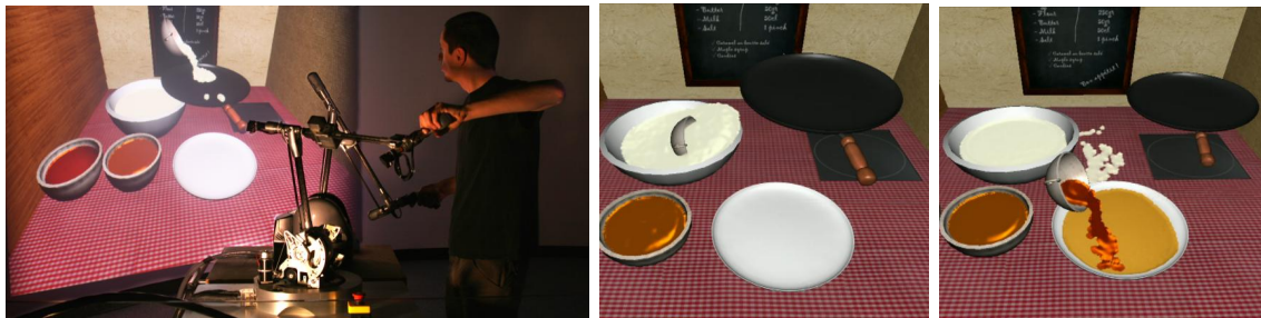
Figure 4.5 – The virtual crepe preparation simulator: the user pours some batter (a high viscosity fluid) from the bowl and into the pan. The user can feel the forces and torques from the pouring movement, as well as the weight shifting between his hands as the batter goes from the bowl to the pan. Maple syrup could also be poured on the crepe.
