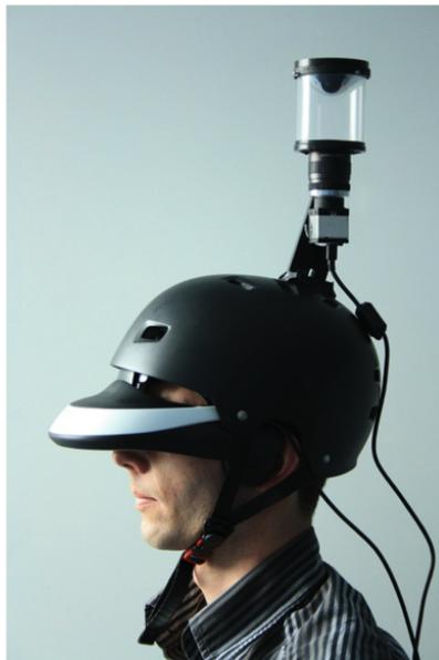
**Figure 8.5** – Illustration of the FlyVIZ prototype.
