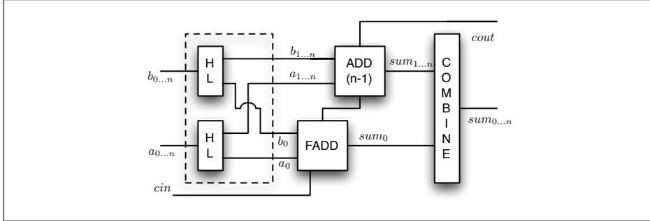
Fig. 1: A recursive  $n$ -bit ripple-carry adder
