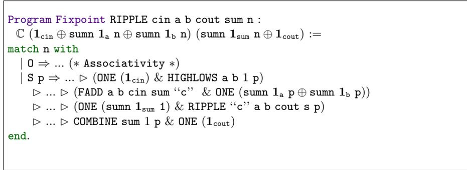
Fig. 7: Implementation of the ripple-carry-adder from Fig. 1
