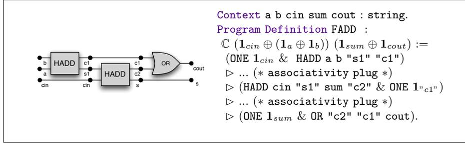
Fig. 6: Definition of a full-adder
