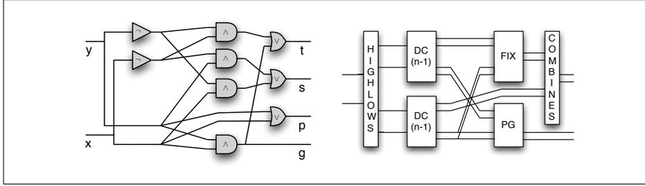
Fig. 8: Divide and conquer adder
