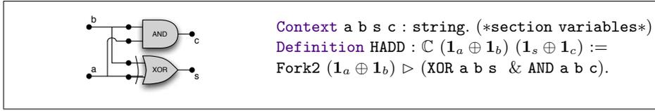
Fig. 5: Definition of a half-adder
