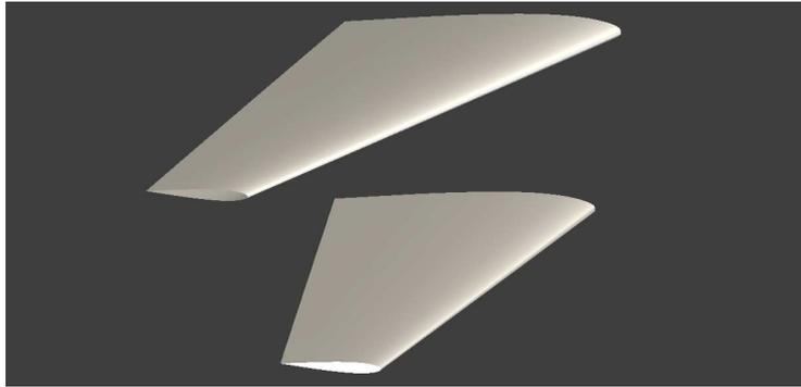
Figure 6: Illustration of sweep angle change.
