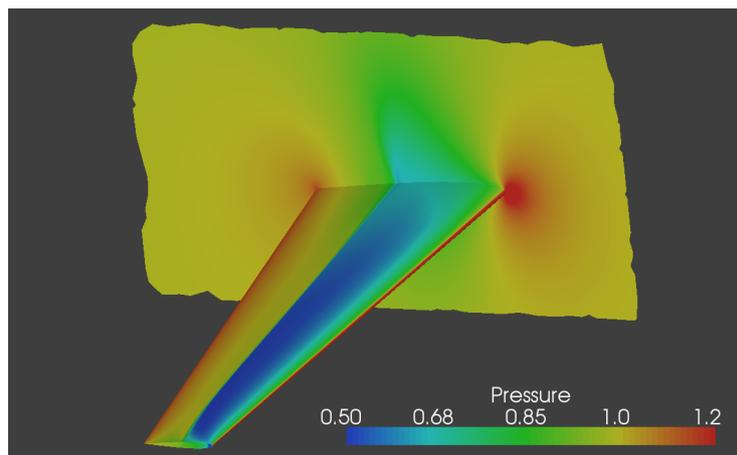
Figure 9: Pressure field for baseline shape.
