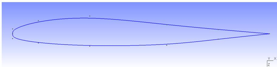
Figure 21: Wing section obtained with successive optimizations approach.
