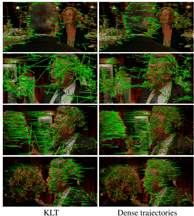
Figure 1. A comparison of the KLT tracker and dense trajectories. Red dots indicate the point positions in the current frame. Dense trajectories are more robust to irregular abrupt motions, in particular at shot boundaries (second row), and capture more accurately complex motion patterns.
