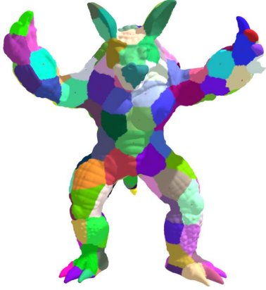
Figure 2. Patches with the Stanford armadillo (173k vertices) with a maximum patch radius of 30.
