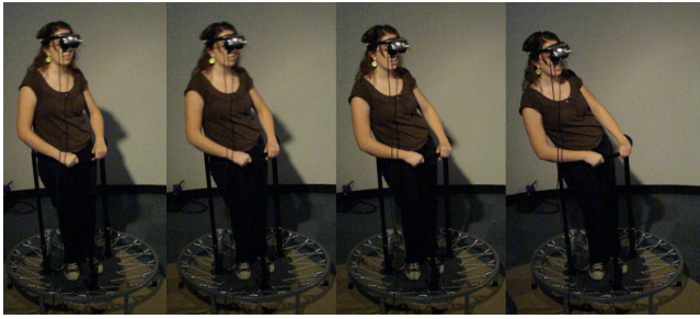
Figure 10: 4 Snapshots extracted from a video sequence acquired during evaluation experiments. We could observe that participants intuitively attempt to use their upper body to control their virtual locomotion in spite of the inefficiency of such actions (note that the platform inclination is almost unchanged from picture to picture). However, this observation provides interesting direction to improve virtual motion controllability, and eventually control side steps from such inputs.
