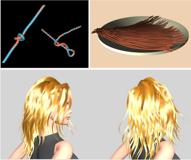
Fig. 2. Various simulations of frictional contact in thin rods. From left to right and top to bottom: interactive formation of a tight knot and a plectoneme, simulation of 76 spaghetti falling in a plate, complex hair contacts with Coulomb friction in wavy hair (84 simulated strands).
