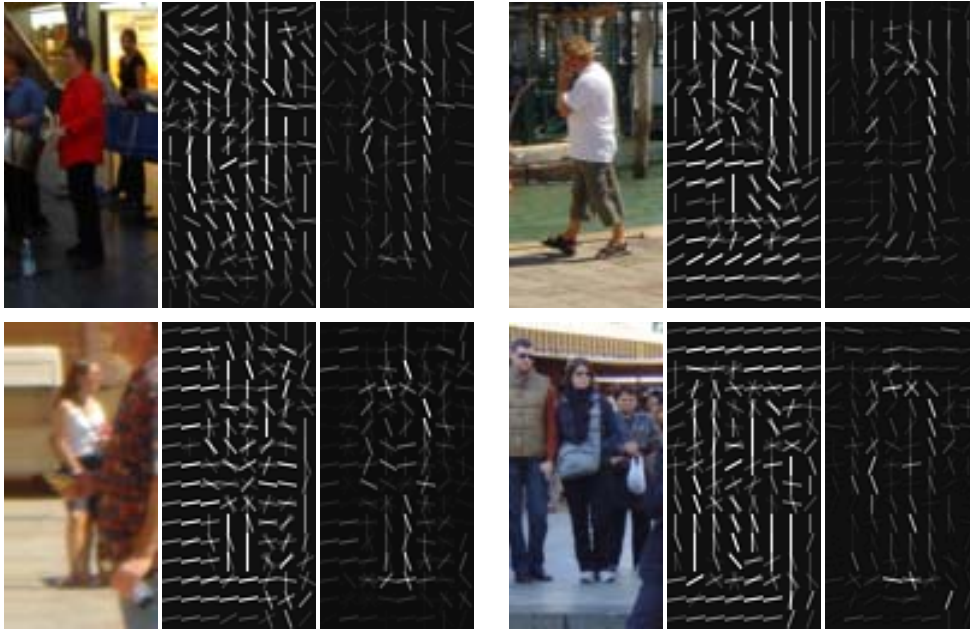
Figure 23: An illustration of the image information encoded by the HOG based detectors. In each triplet, we display from left to right: (1) the input image; (2) the corresponding HOG feature vector (only the dominant orientation of each cell is shown); (3) the orientations that dominate the descriptor output (obtained by multiplying the feature vector with the weights learned for the linear SVM). Inspection shows that for an appropriate choice of descriptor parameters, the SVM is able to map positive example images to a set of canonical edges corresponding to human contours.
