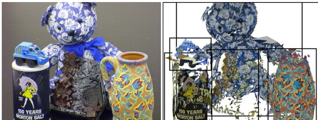
Figure 19: Results of a recognition experiment. Left: A test image. Right: Instances of five models (a teddy bear, a doll stand, a salt can, a toy truck and a vase) have been recognized, and the models are rendered in the poses estimated by our program. Bounding boxes for the reprojections are shown as black rectangles.
