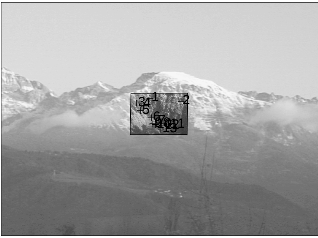
Figure 4. The high-resolution image is mapped onto the low-resolution one using the homography consistent with 13 point-to-point assignments.
