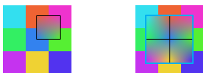
Figure 6: Interpolation cells (left, black square) for bilinear magnification mode are dual to the texel grid i.e. their corners are placed at texel centers. The influence area of the center texel (right, blue square) is the union of the four interpolation cells requiring the texel.
