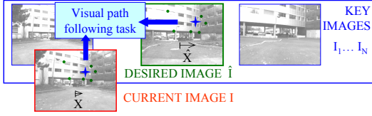
Fig. 2. The current and desired images contain some common visual features, which are used for navigation.
