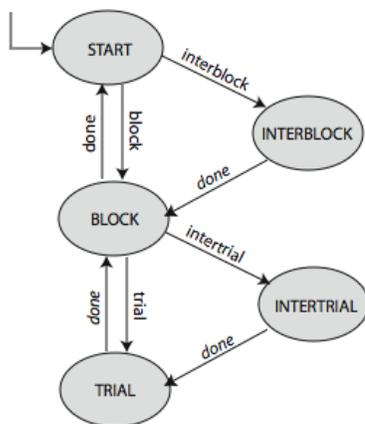
**Figure 8. State Machine running the experiment**
