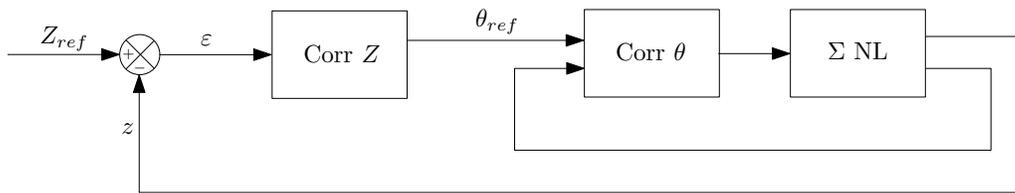
Figure 33: New cascade structure for the AUV control
