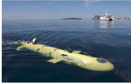
Figure 22: The *Aster<sup>X</sup>* AUV operated by Ifremer
