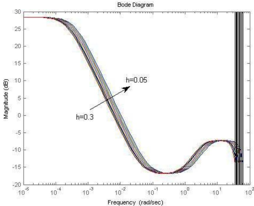
Figure 26: Bode diagram of the LPV/LFT controller
