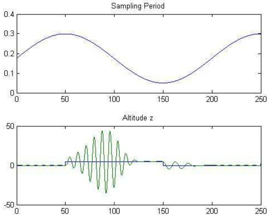
Figure 30: altitude  $z$  with discrete-time  $\mathcal{H}_\infty$  controller,  $h$  sinusoidal
