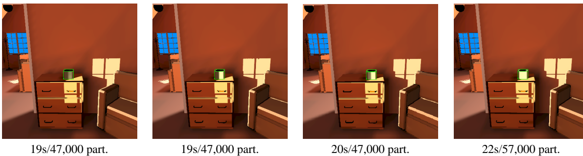
Figure 7: Four positions of the container on the dresser in the bedroom, the update times are shown beneath each image. Note the increase in brightness on the container and the moving shadow behind
