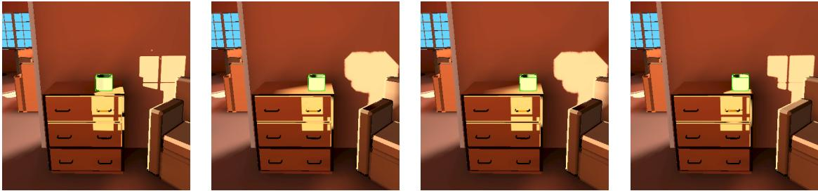
**Figure 5:** (Left) Initial position with good quality shadow. (Middle) two intermediate positions during degraded quality motion at 3-4 sec/frame. (Right) Motion has ended, 20 seconds later we obtain the quality shown, equivalent to normal updates.
