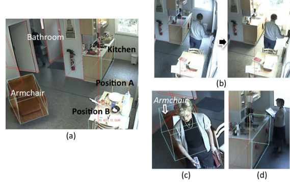
Figure 12. (a) Example of scene logical regions. (b) The person turns on the kitchen light producing a change of the illumination that leads to a tracker mistake. (c) The camera perspective confuses the person “Standing” as if it is “Sitting at the armchair”, (d) The motion of the person while it is “reading a magazine” at the kitchen is confused with the activity “Cooking”.
