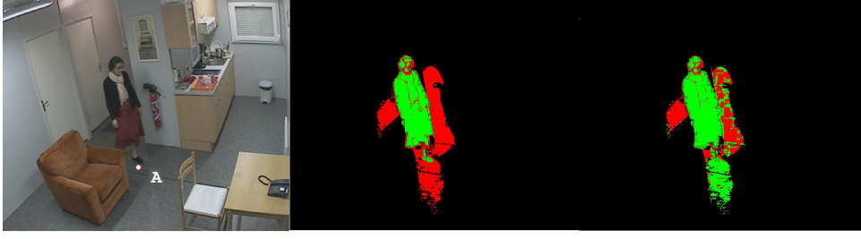
Figure 2. Shadow detection results using normalized RGB color space (center image) and HSV color space (right image) as in [6]. Red regions correspond to detected shadow regions. In RGB color space, the luminance of pixel A when there is shadow is (71,75,74) and when there is no shadow is (90,91,86). In HSV color space, this two values correspond to (H = 165, S=5%,V = 29%) and (H = 72, S = 5%,V = 36%), a big difference in hue.
