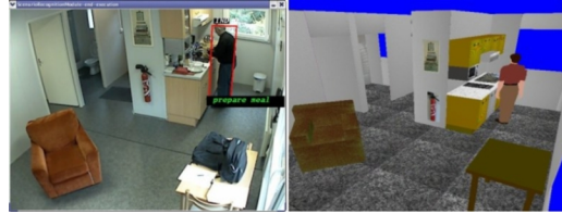
Figure 5. (a) Recognition of "preparing a meal" activity. (b) the 3D visualization of this recognition.
