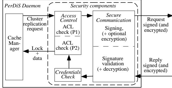
**Figure6.** Security operations when requesting a cluster copy
