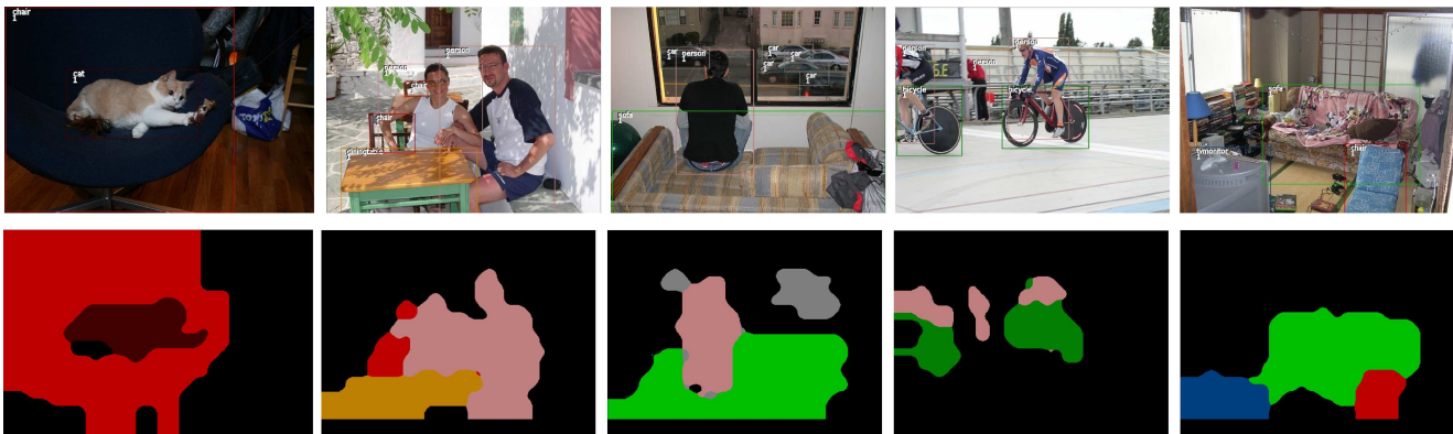
Fig. 11 Examples of additional annotations (segmentation masks) automatically produced for the unsegmented training images, obtained by applying our algorithm on the provided bounding boxes (best viewed in color, with color coding shown in Figure 13).
