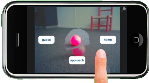
Fig. 6. When a joint attention situation has been achieved on an object, a set of actions are presented to the user, which can in particular decide to teach a name for this object
