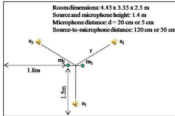
Figure 3: Room geometry setting for synthetic convolutive mixtures.
