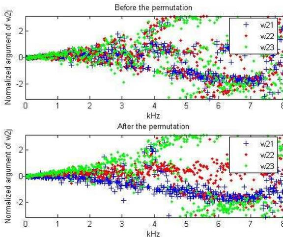
Figure 2: Normalized argument of  $w_{2j}(f)$  before and after permutation alignment from a real-world stereo recording of three sources with  $RT_{60} = 250$  ms.
