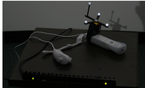
Figure 18: Optically tracked Nintendo wiimote
