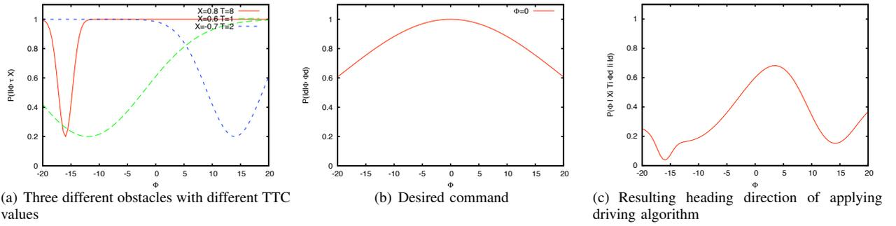
Fig. 3. Example of the Gaussian Driving algorithm involving the computation of the heading direction in the presence of three different obstacles with different TTC values.
