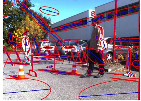
Fig. 2. An example of Scale Invariant Ridge Segments detection. Each detected segment is represented by an ellipse where the main axis represents the position of the segment and the second axis represents the scale.
