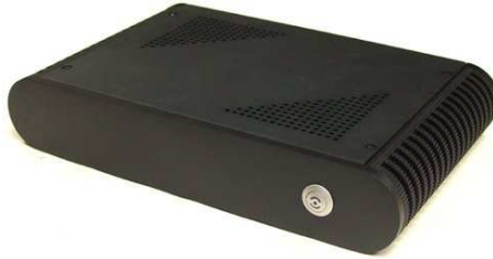
Figure 1: Neo CI852A-4RN10 barebone used for the DSLnodes.
