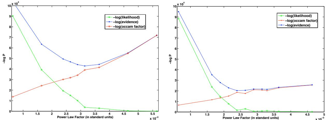
Figure 8: *Evidence maximization w.r.t energy flux.* Minus log of evidence (blue), likelihood (green) and Occam factor (red) v.s. power law factor  $\beta$  (i.e. energy flux  $\epsilon$ ) for horizontal winds at low (*left*) and at intermediate (*right*) altitude
