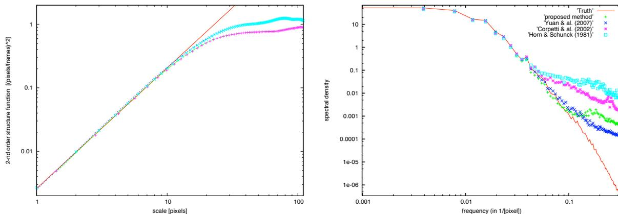
Figure 5: **2-nd order statistics.** *Left* : Power law maximizing evidence (continuous red line). True (dash line) and estimated (crosses) 2-nd order structure functions in horizontal-vertical (in blue and turquoise) and diagonal (in pink and green) directions . *Right* : Energy spectra  $E(k)$  of first order (in turquoise), div-curl (in blue or pink) and self-similar (in green) regularizers compared to the true (in red) spectrum.
