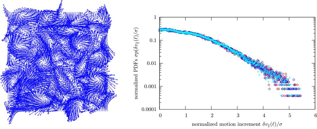
Figure 1: *Bidimensional turbulent motion and similarity through scales of the normalized motion increment PDFs  $\sigma_\ell p_\ell(\frac{\delta v_{\parallel}(\ell)}{\sigma_\ell})$  for scale increment  $\ell = 1, 2, 4$ .*
