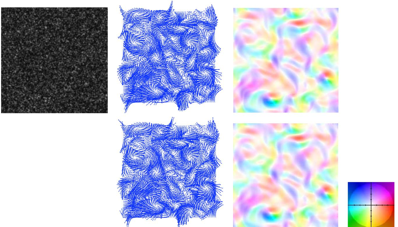
Figure 2: *Bidimensional turbulence. Above. Particle image at initial time (left). True velocity field (middle) and its scalar (right) representation. Below. Estimated velocity field (middle) and its scalar (right) representation together with (Baker et al., 2007) color system for scalar visualization of vector fields.*
