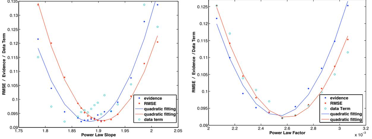
Figure 3: **Scaling model selection.** Behavior of data term and minus the evidence logarithm w.r.t slope  $\zeta$  (*left*) and factor  $\beta$  (*right*) in comparison to the RMSE. For comparison, evidence and data term ranges of value have been rescaled on the RMSE.
