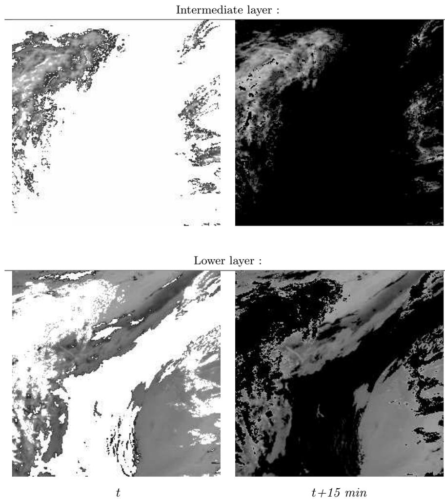
Figure 7: **Input meteorological images.** Sparse pressure difference maps of layers at intermediate (above) and low (below) altitude. White pixels of image at time  $t$  and black pixels at time  $t + 15$  minutes are areas with no observations. The images characterize the layers evolution in a time interval of 15 minutes.
