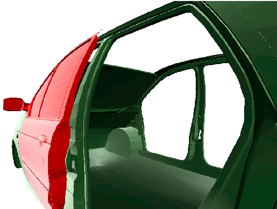
Figure 5. Third test application: the door being interactively positioned in the car skeleton. Continuous collision detection and constraint-based simulation allows the user to precisely and intuitively position the door. No interpenetration ever occurs.
