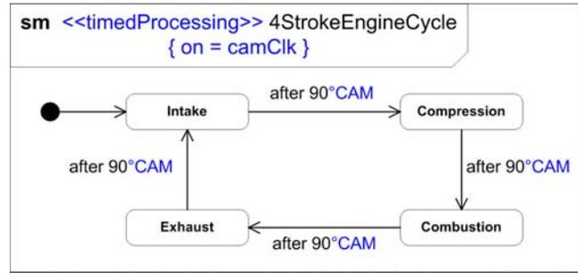
Figure 10. A state machine with multiform time
