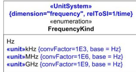
Figure 6. Identify units for the dimension frequency
