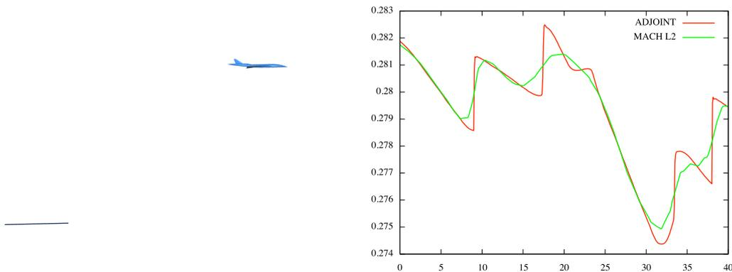
Figure 4: *3D supersonic aircraft simulation. Left, position of the observation plane with respect to the aircraft. Right, comparison of the pressure in the observation region between the goal-oriented (red) and the multi-scales (green) mesh adaptations for the same mesh size.*
