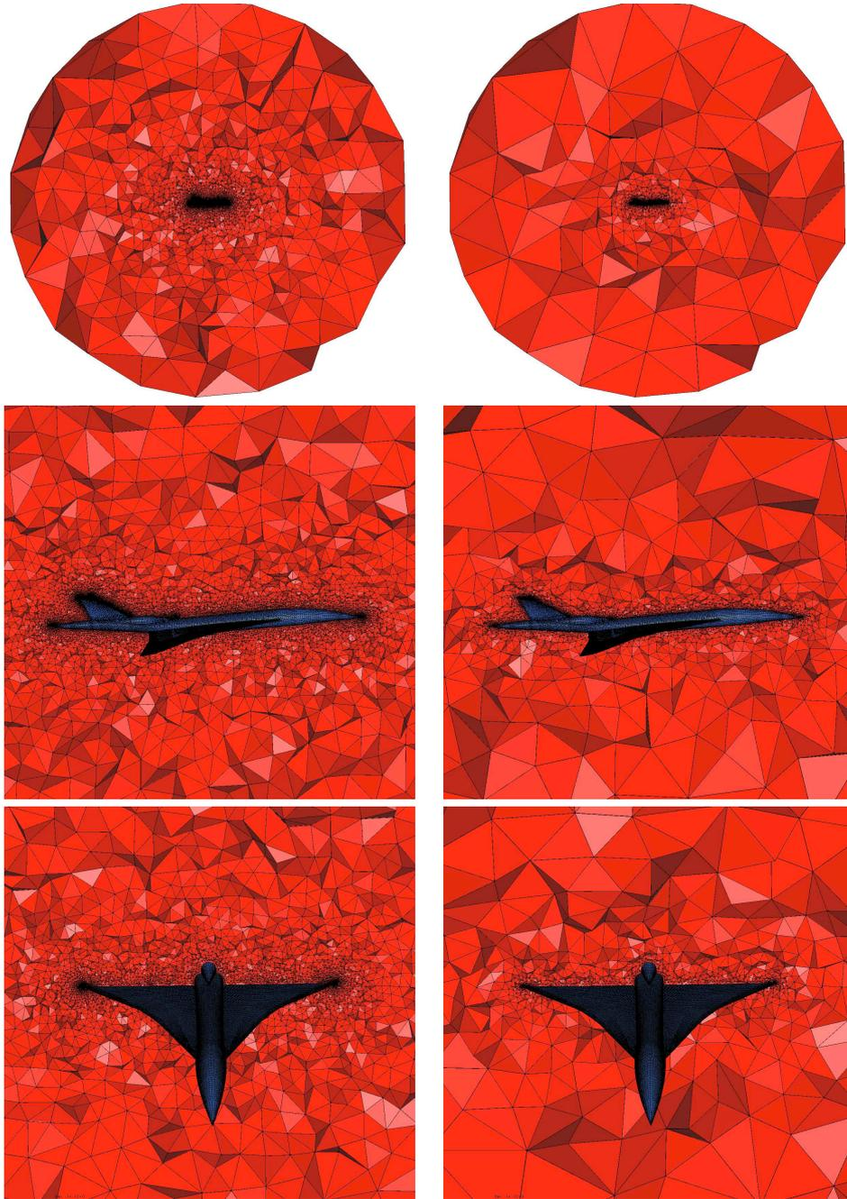
Figure 12: *Graded isotropic mesh of an aircraft in a spherical domain. Left, the mesh for a size gradation of 1.2 containing 3,574,143 tetrahedra. Right, the mesh for a size gradation of 1.5 containing 946,236 tetrahedra.*
