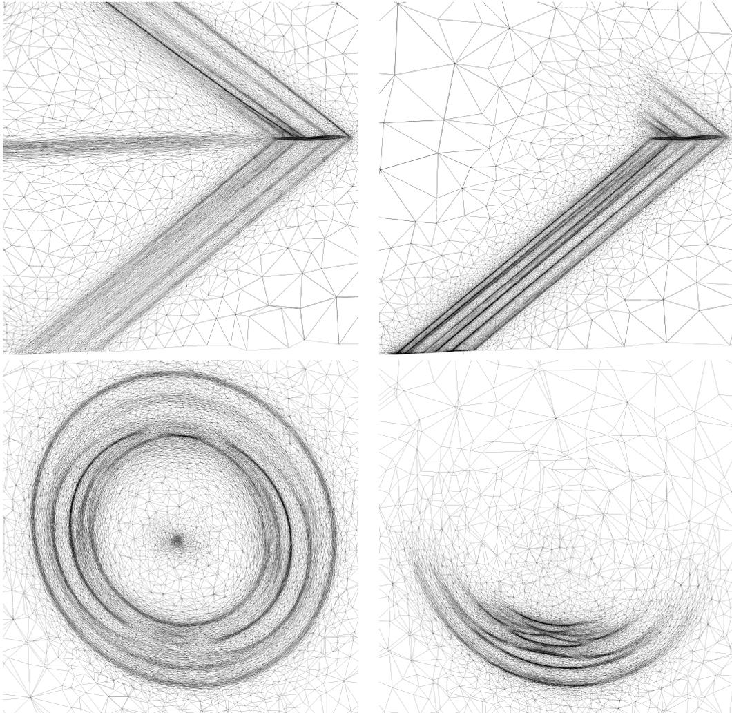
Figure 5: *3D supersonic aircraft simulation. Left, the final anisotropic mesh with the multi-scales mesh adaptation in  $L^2$  norm. Right, the final anisotropic mesh with the goal-oriented mesh adaptation.*
