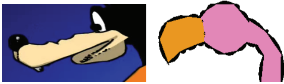
Figure 2: Using rasterization to define filled regions can yield aliasing artifacts, as shown in Goofy's lower lip rendering with Swift3D (left) and the flamingo's beak/head intersection rendered by LiveArt.
