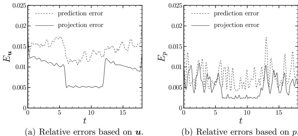
Fig. 5. Comparison of the prediction and projection relative errors based on  $\mathbf{u}$  and on  $p$  for the controlled cylinder wake flow ( $\gamma(t) = A \sin(2\pi S t_f t)$  with  $A = 2$  and  $S t_f = 0.5$ ). The approximations  $\hat{\mathbf{u}}$  and  $\hat{p}$  are evaluated for  $N_{\text{gal}} = 14$ .
