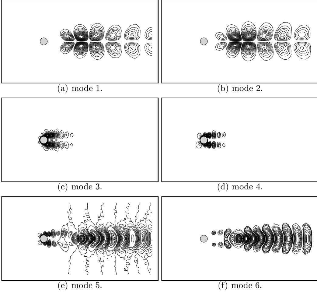
Fig. 4. Pressure POD basis functions for the controlled cylinder wake at  $Re = 200$ . The first six POD modes  $\phi_n^p$  are visualized by iso-contour lines of their norm ( $\|\phi_n^p\|_\Omega$ ) for  $\gamma(t) = A \sin(2\pi St_f t)$  with  $A = 2$  and  $St_f = 0.5$ .
