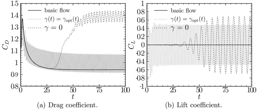
Fig. 12. Time evolutions of the aerodynamic coefficients for the basic flow (solid line), uncontrolled flow ( $\gamma = 0$ , dashed lines) and optimally controlled flow ( $\gamma(t) = \gamma_{\text{opt}}(t)$ , dotted lines). Control was started at time  $t = 0$ .
