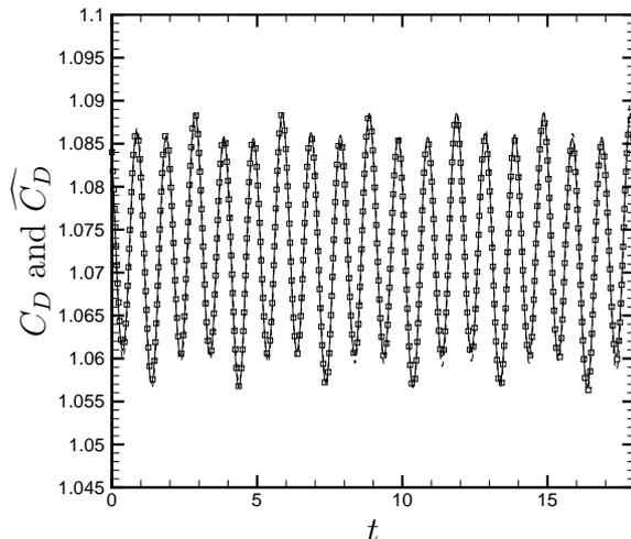
Fig. 7. Comparison of the real drag coefficient  $C_D$  (symbols) and model function (lines) of the drag coefficient for the controlled cylinder wake flow ( $\gamma(t) = A \sin(2\pi St_f t)$ ) with  $A = 2$  and  $St_f = 0.5$ .
