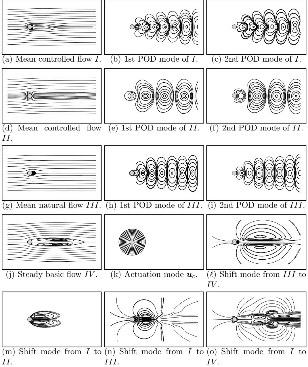
Fig. 6. Modes considered in the reduced-order control model (12) of the cylinder wake at  $Re = 200$ . In all sub-figures, the flow is visualized with streamlines. Note that subfigure 6(d) looks like a potential solution and that subfigure 6(k) approximates a potential vortex.
