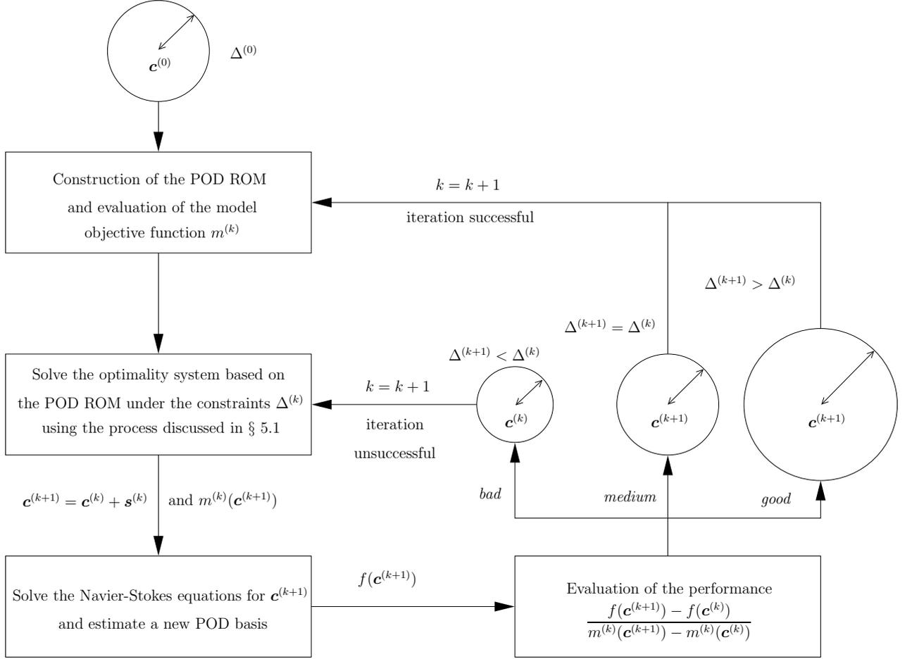
Fig. 3. Schematic representation of the TRPOD algorithm.
