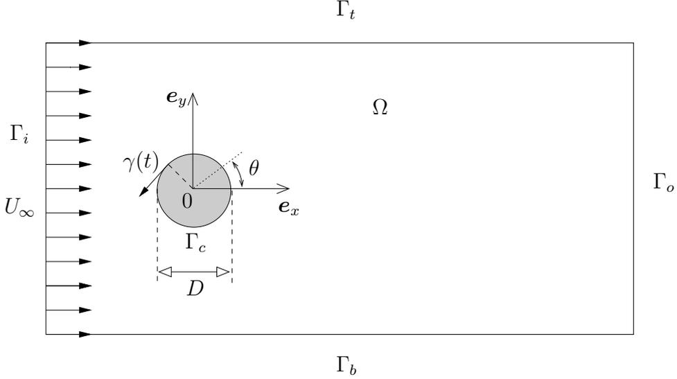
Fig. 1. Controlled flow configuration.
