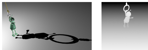
Figure 8: Shadow map for a point light source. Left: view from the camera. Right: depth buffer computed from the light source.
