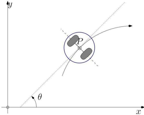
Fig. 1: Model of a differential drive robotic system.
