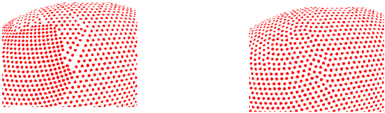
Figure 5 Illustration of the relaxation process. (left) After the generation holes can appear. (right) After the relaxation all holes have disappeared.
