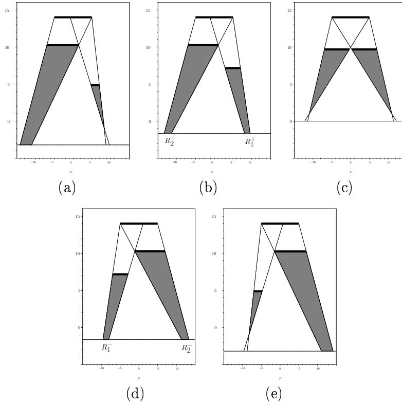
Figure 6: Views in the sweep plane with bitangents that define the umbra. The number of components of umbra in the intersection of the sweep plane and the plane  $z = 0$  is : (a) one (sweep plane through  $(0, 10, 0)$ ), (b) two (sweep plane  $P_+$  through  $(0, 7, 0)$ ), (c) zero (sweep plane  $y = 0$ ), (d) two (sweep plane  $P_-$  through  $(0, -7, 0)$ ), (e) one (sweep plane through  $(0, -10, 0)$ ).
