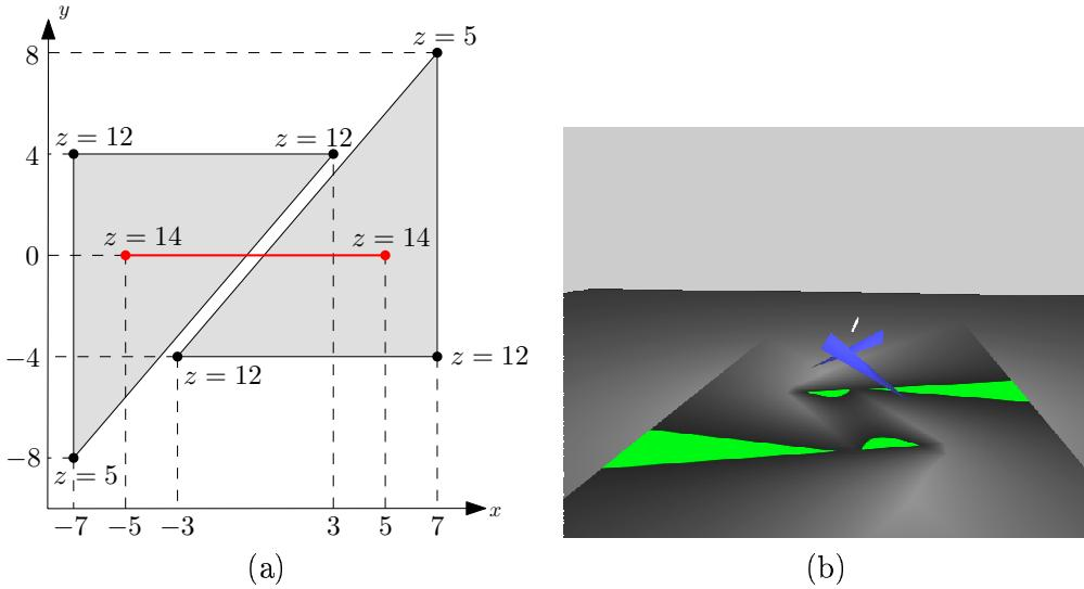
Figure 4: (a) Two triangles and a segment light source (viewed from above) that cast 4 connected components of umbra on the plane  $z = 0$ . (b) The scene rendered with the ray tracer OpenRT (the umbra is in light grey); courtesy of Andreas Dietrich.
