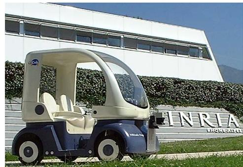
**Fig. 10.** the cycab: an autonomous car-like robot platform
