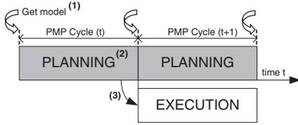
**Fig. 2.** Partial Motion Planning architecture
