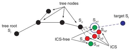
**Fig. 4.** Tree construction over a PMP cycle
