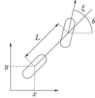
Fig. 1. The car-like vehicle  $\mathcal{A}$  (bicycle model).
