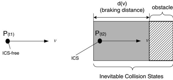
**Fig. 3.** Inevitable Collision State vs. Safe State
