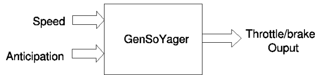
Fig. 2. The throttle/brake subsystem scheme
