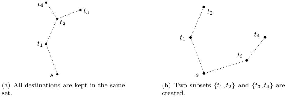
Figure 3: The message splitting strategy used by MSTTEAM:  $\Delta(s, t_1, t_2, t_3, t_4)$  is used to split the message at node  $s$ .
