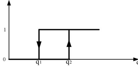
**Fig. 5:** Double Thresholds Control Function of the Switch
