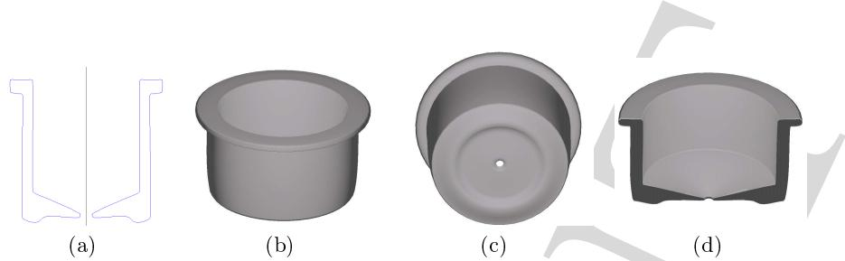
**Fig. 9.** Creation of a flowerpot. This model was designed with the profile curve shown in (a) combined with a circular silhouette curve. (b) and (c) show the pot from different points of view while (d) presents a cut-view. Note that the pot is actually a genus 1
