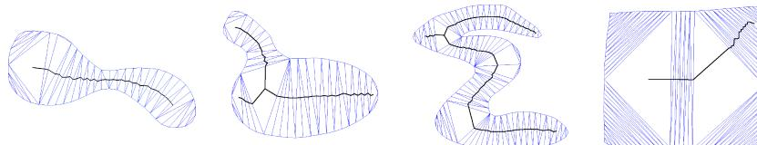
**Fig. 15.** CDT of different silhouette curves. We can see the skeletons discontinuities.
