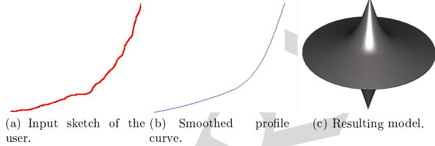
**Fig. 6.** From the input profile curve to the resulting 3D model.
