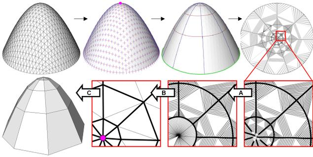
Figure 8: *Remeshing phase: a dome-like shape is sampled with lines of curvatures. All the curvature line segments (red/blue) and the feature edges (green) are added as constraints in a CDT in parameter space. The CDT creates a dense triangulation; a rapid vertex decimation (A,B) then suppresses most small edges, and leaves only few vertices, defining a coarse polygonal mesh. Adding constraint edges to the umbilic (center) point takes care of the near-spherical cap.*
