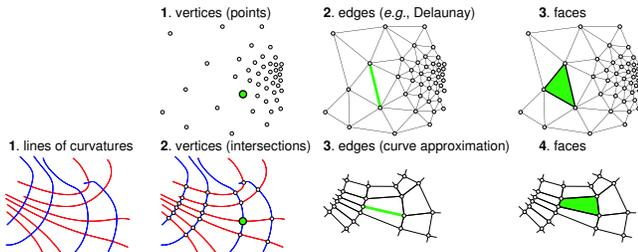
Figure 7: *Point-based sampling vs. curve-based sampling: while most techniques spread vertices first before deducing edges and faces, we use lines of curvatures on anisotropic areas to find vertex positions, before simplifying these lines to straight edges, and then deducing faces. Note that we use regular point-sampling on nearly-isotropic areas since principal directions are meaningless when the surface is almost spherical.*
