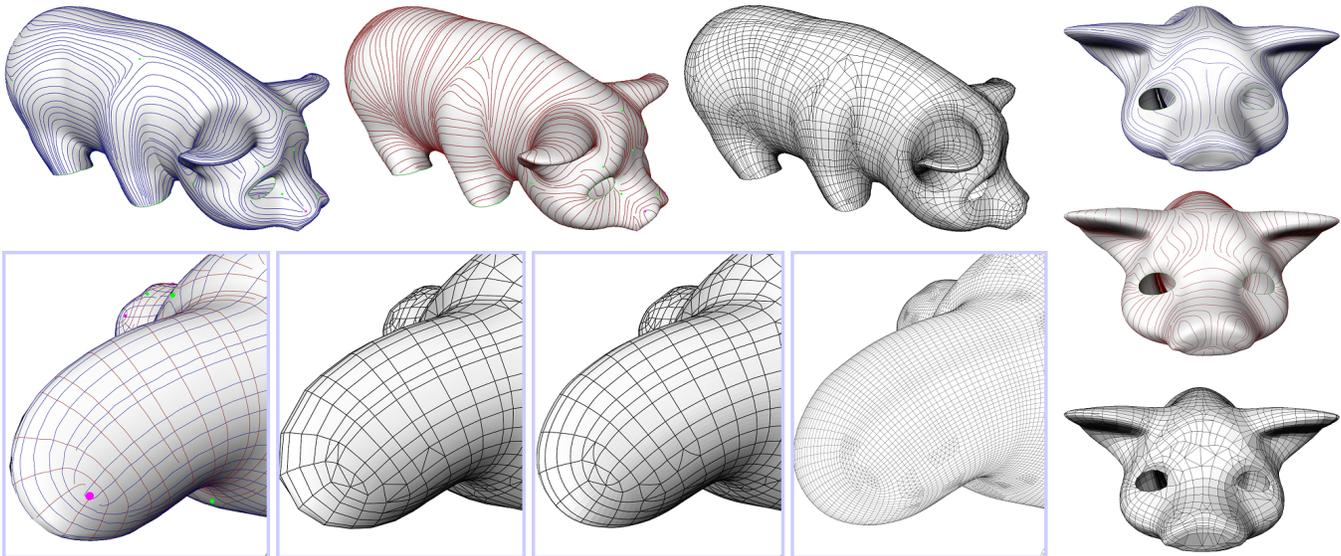
Figure 11: *Remeshing a pig. Row 1, and right column: lines of minimum (blue) and maximum (red) curvature, and the anisotropic polygon mesh generated. Row 2: close-up on an ear showing the lines of curvatures, the resulting polygon mesh with conforming edges, the surface after quad/triangle subdivision (edges of the coarse model are superimposed), and the mesh after two iterations of subdivision.*
