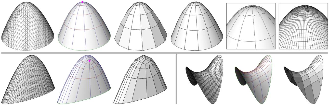
Figure 10: *Top: A dome-like shape, its lines of curvatures, the output of our remeshing process, its limit surface after quad/triangle subdivision, with two close-ups of the cap; Bottom: A squeezed dome and a saddle shape exhibit high anisotropy.*
