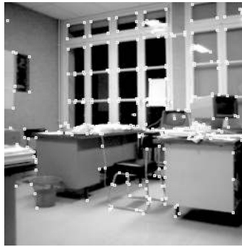
Figure 11: Junctions extracted at the zero-crossings of the Laplacian of Gaussian .
